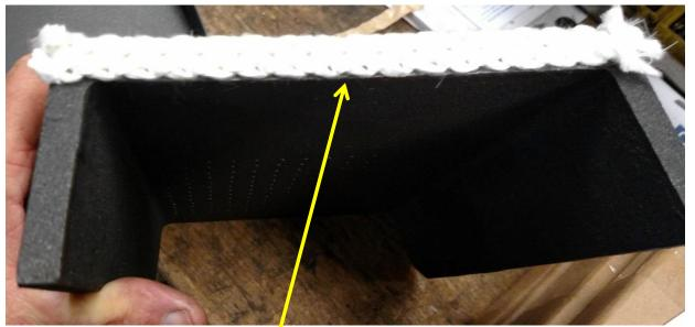
Verify grate firmly seats against feeder frame and gasket is flush with feeder frame and grate.
