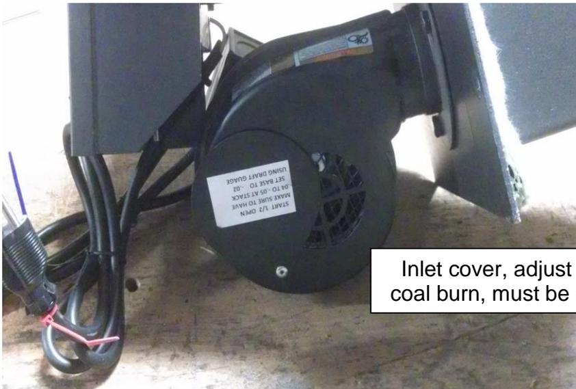
Inlet cover, adjust to obtain proper coal burn, must be open at least half
