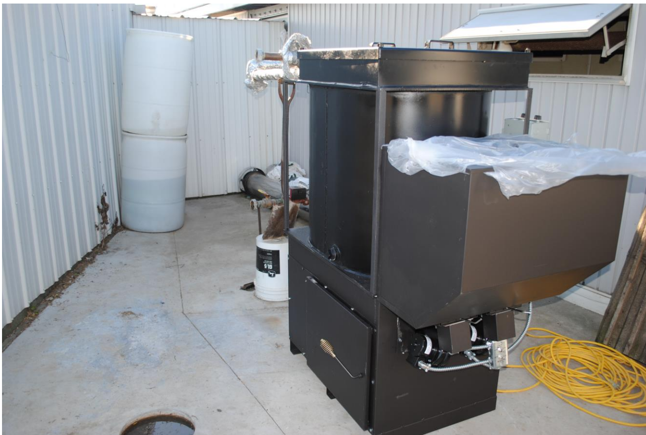
Assembled boiler without jacket and insulation
